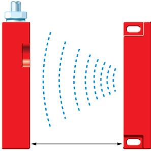
Encapsulated in the MA Series is a unique high-power industrial reed which is de-rated by a non-resettable overload protection circuit depending on switch type. On presenting the actuator to the switch, the high intensity magnetic field from the actuator causes the contacts to close. On removing the actuator (opening the door), the safety contacts open, isolating the machine.
