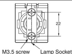
Note: The figure shows an example of the terminal arrangement when the Socket Unit is removed.
