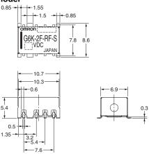
Note 1. Each value has a tolerance of ±0.3 mm. Note 2. The coplanarity of the terminals is 0.15 mm max.
