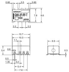
**Mounting Dimensions** (Top View) Tolerance: ±0.1 mm
