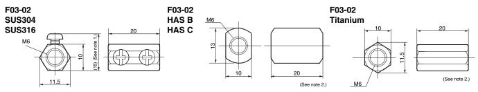
Note: 1. Dimension when mounting Electrodes.
