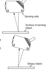
• If there is a mirror-like object below the Sensor, the Sensor may not operate stably. Therefore, incline the Sensor or separate the Sensor from the mirror-like object as shown below.
