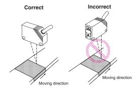
• The stability indicator may turn off in reaction to reflection from background objects. In such cases, incline the Sensor by  $10^{\circ}$  as shown in the illustration for more stable detection.
