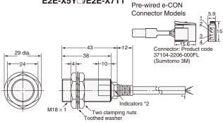
\*1. 6-dia. vinyl-insulated round cable with 2 conductors (Conductor cross section: 0.5 mm²,
