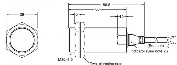
**Note 1.** 4-dia. vinyl-insulated round cable with 3 conductors (conductor cross section: 0.3 mm<sup>2</sup>; insulator diameter: 1.3 mm); standard length: 2 m
