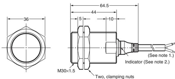
Note 1. 4-dia. vinyl-insulated round cable with 3 conductors (conductor cross section: 0.3 mm<sup>2</sup>; insulator diameter: 1.3 mm); standard length: 2 m
