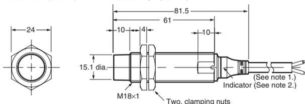
**Note 1.** 4-dia. vinyl-insulated round cable with 3 conductors (conductor cross section: 0.3 mm<sup>2</sup>; insulator diameter: 1.3 mm); standard length: 2 m
