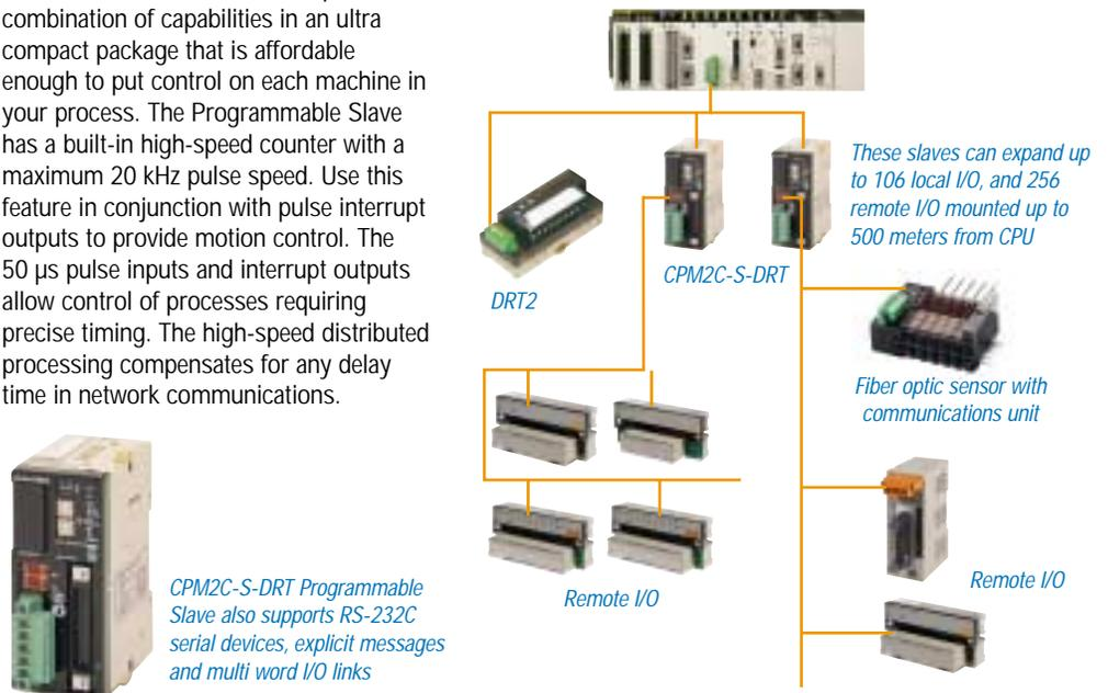
CPM2C-S-DRT Programmable Slave also supports RS-232C serial devices, explicit messages and multi word I/O links
