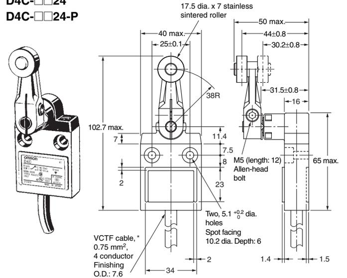
\* S-FLEX VCTF Cables are used for weather-resistant models.
