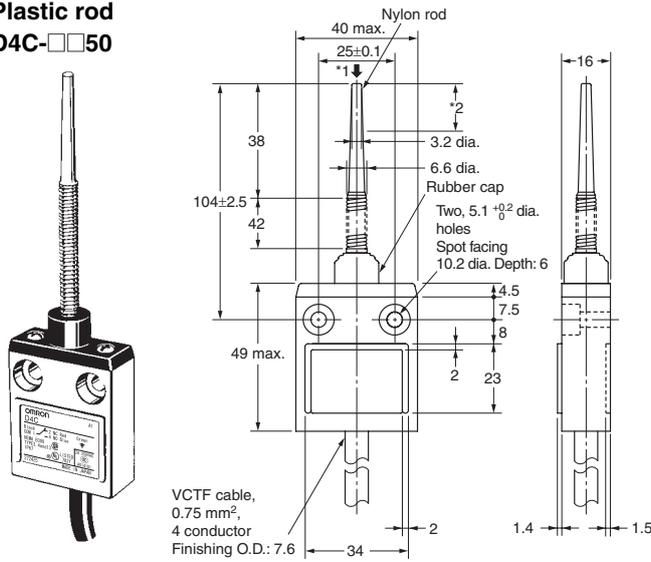
\*1 Operation is possible in any direction except in parallel to the axis.
