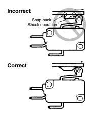
Make sure that no improper force is applied to the actuator, otherwise the actuator may incur local abrasion. As a result, the actuator may become damaged or its durability may be deteriorated.
