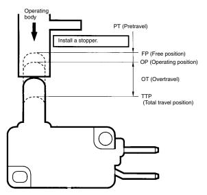
If stroke is set in the vicinity of the operating position (OP) or the releasing position (RP), contact force may become unstable. As a result, the switch cannot ensure high reliability. Furthermore, the switch may malfunction due to vibration or shock.
