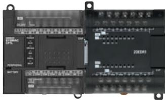
Note: CP1L (L Type) CPU Units with 10 points do not support Expansion Units.
