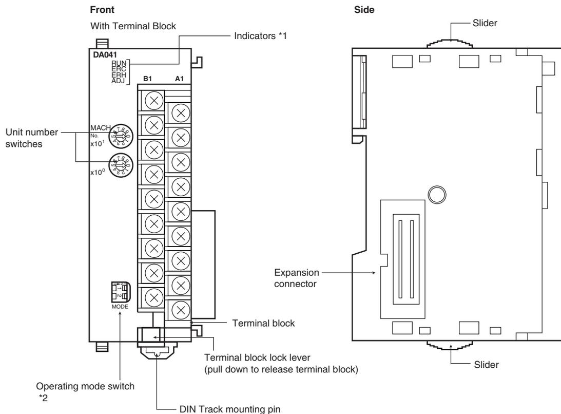
\*1 The ADJ LED is not provided with the CJ1W-DA042V.
