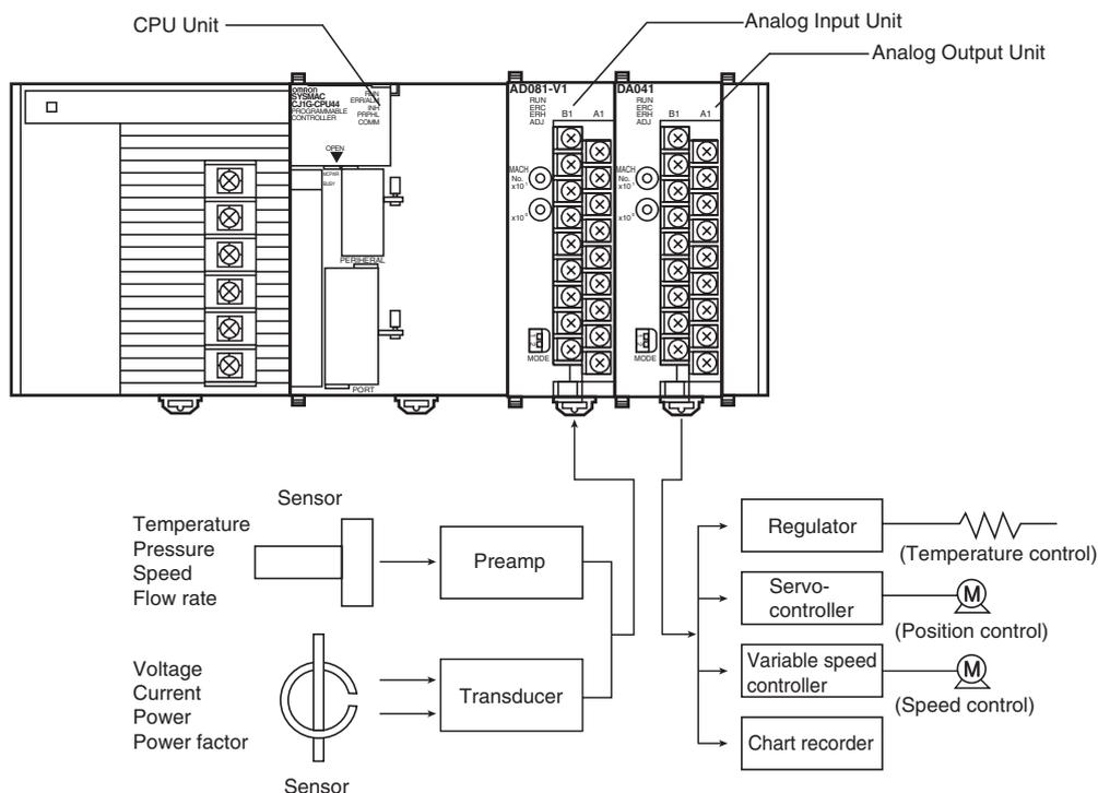
**Note:** The above diagram is an installation example for the CJ1W-AD081-V1 Analog Input Units and CJ1W-DA041 Analog Output Units.
