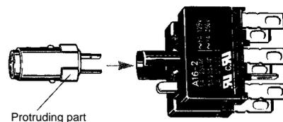
The Lamp can be mounted from the operating part end by using the A16Z-5080 Extractor. The lamp can be mounted by following the opposite procedure for removing the Lamp.
