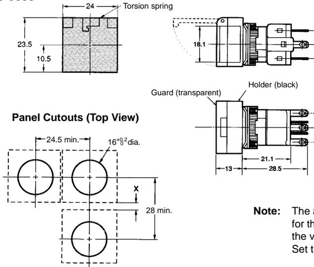
**Note:** The above illustration shows a case where 4.5 mm is provided for the distance "x." If no clearance is required for the "x" section, the vertical mounting dimension can be as small as 24 mm. Set this distance according to operating conditions.
