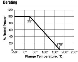
Limitation obtained by actual test with 0.01 duty continuous pulse repetition for TGHMV10R0JE, four times safety factor was considered. Please note this is not a specification, this is a typical data.
