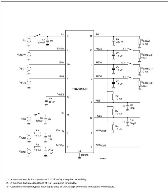
Fig.8 Test circuit.
