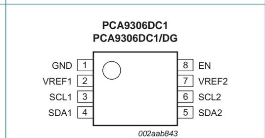
Fig 5. Pin configuration for VSSOP8 (DC1; DC1/DG)
