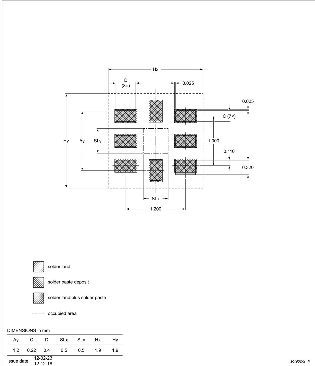
Fig 29. PCB footprint for SOT902-2 (XQFN8); reflow soldering
