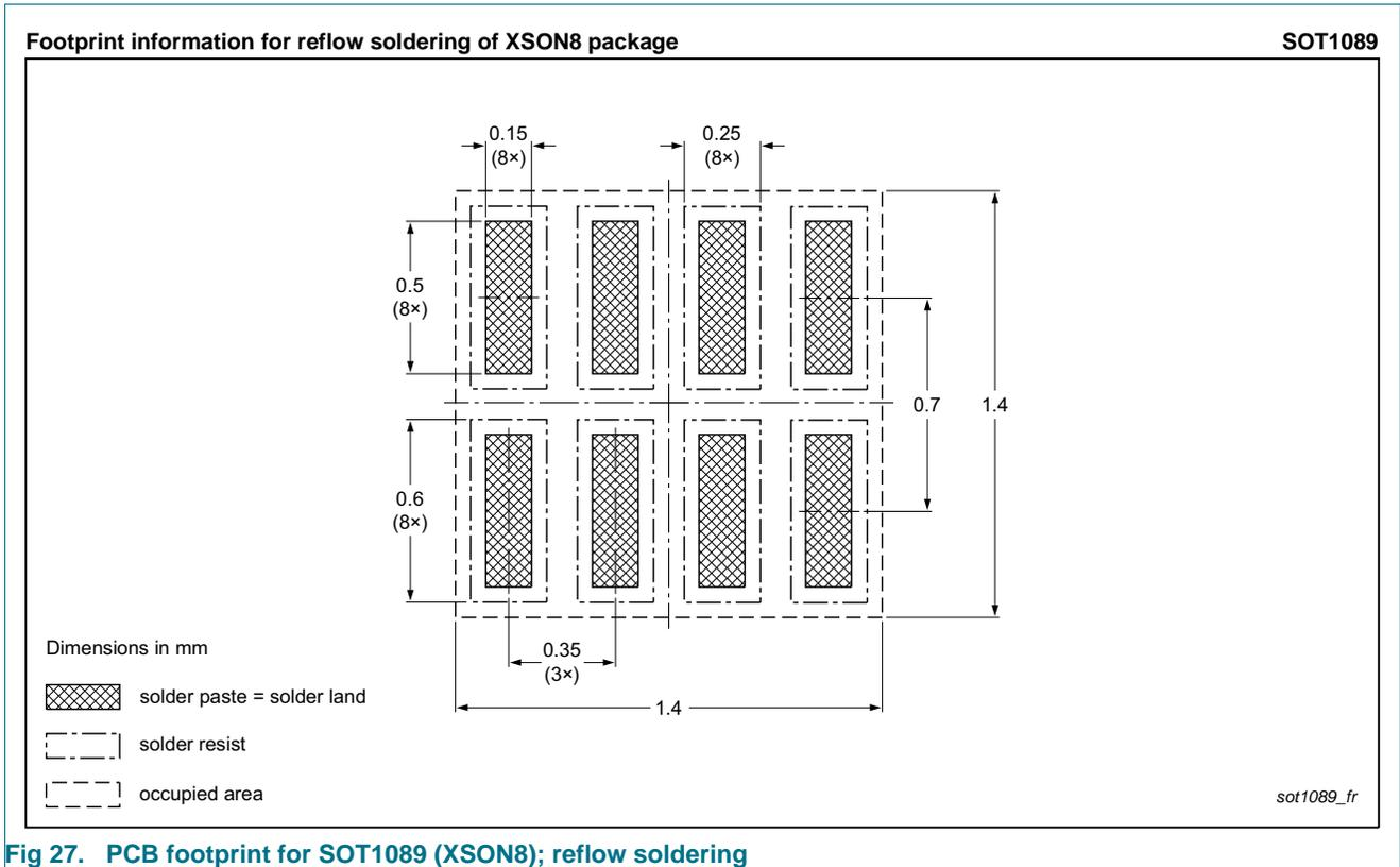
**Fig 27. PCB footprint for SOT1089 (XSON8); reflow soldering**
