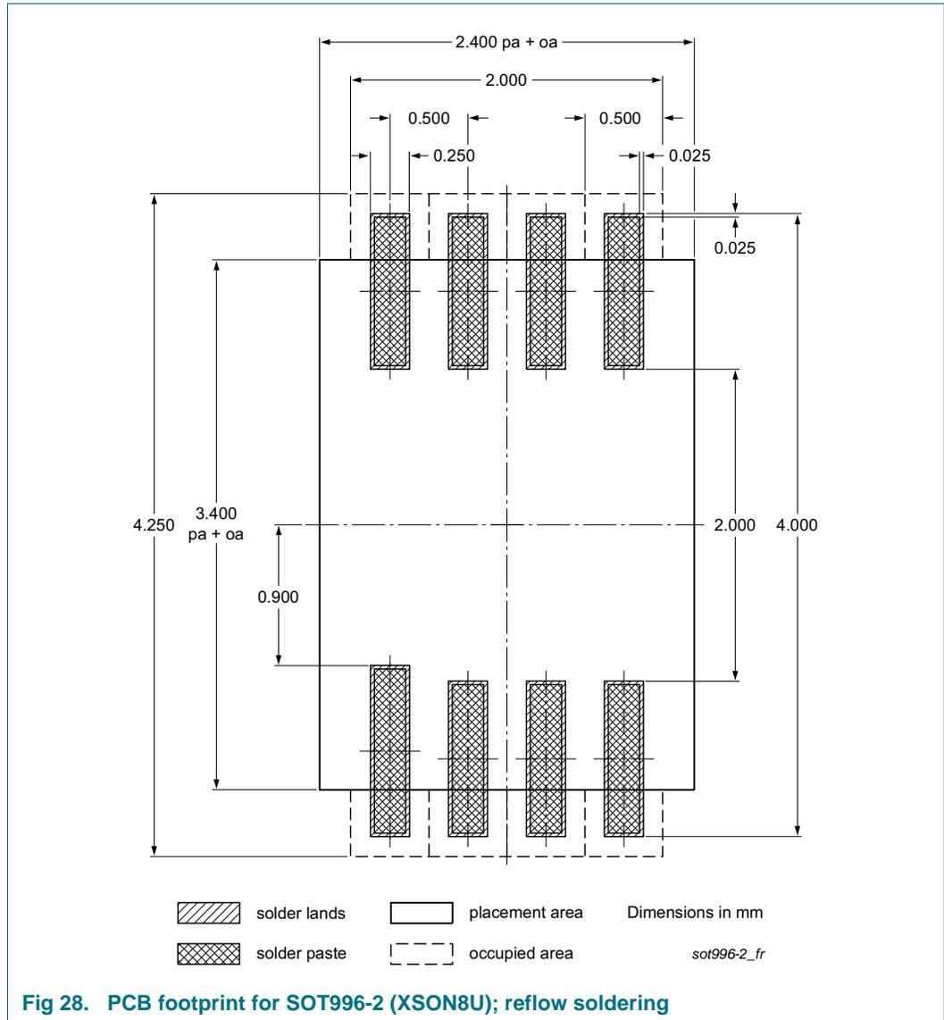
Footprint information for reflow soldering of XQFN8 package
