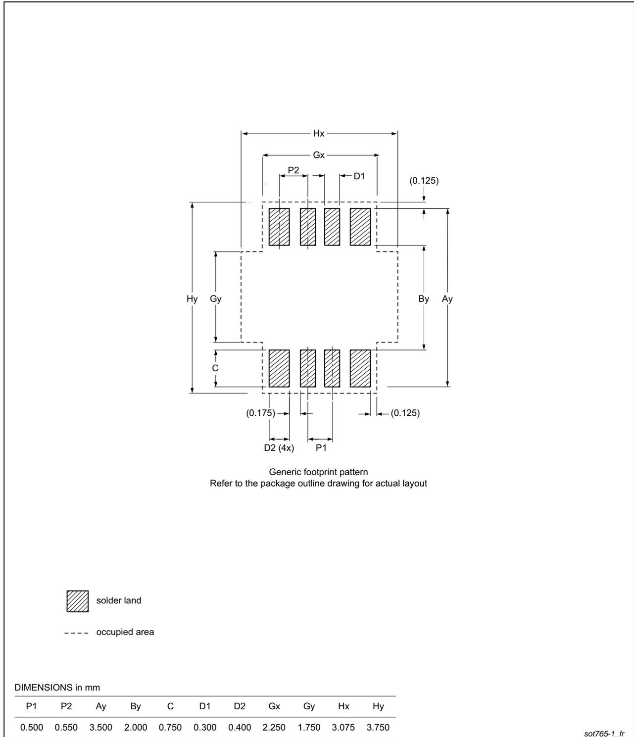
Fig 26. PCB footprint for SOT765-1 (VSSOP8); reflow soldering
