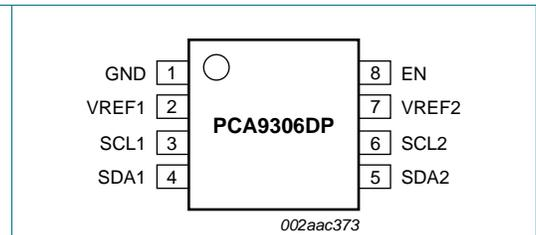
Fig 3. Pin configuration for TSSOP8 (DP) (MSOP8)
