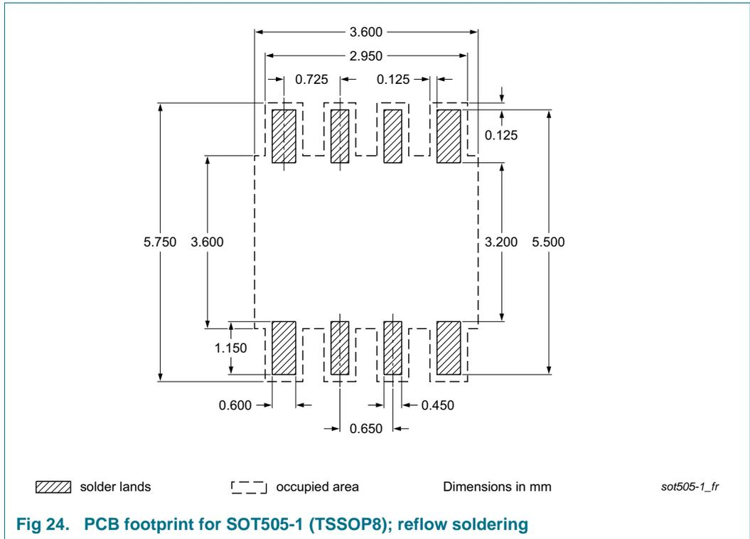
Footprint information for reflow soldering of TSSOP8 package
