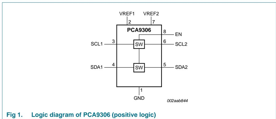
Fig 1. Logic diagram of PCA9306 (positive logic)
