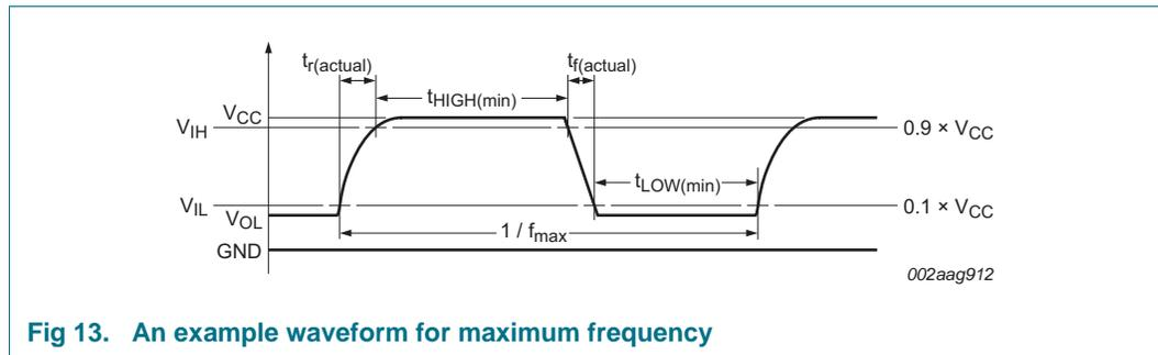
Fig 13. An example waveform for maximum frequency
