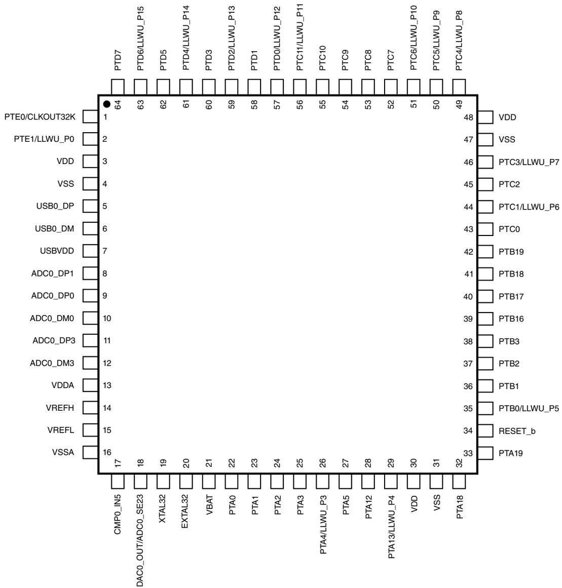
Figure 7. 64 LQFP Pinout Diagram
