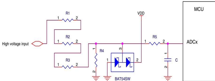
**Figure 42. High voltage measurement with an ADC input**
