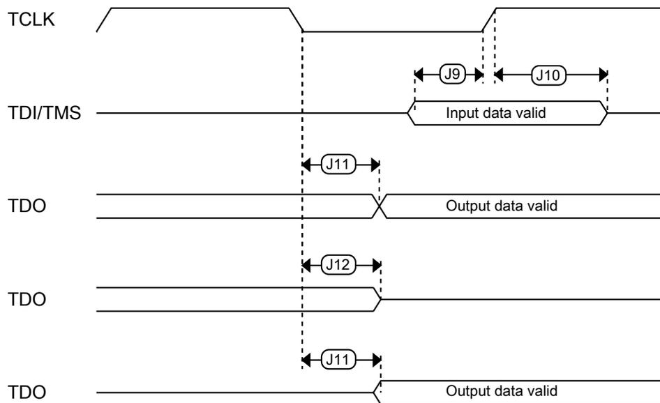
Figure 22. Test Access Port timing
