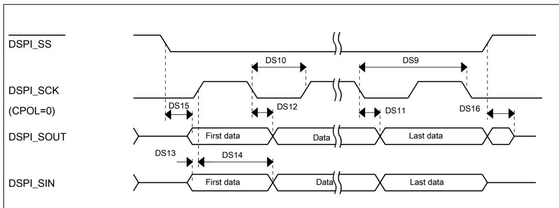
**Figure 34. DSPI classic SPI timing — slave mode**
