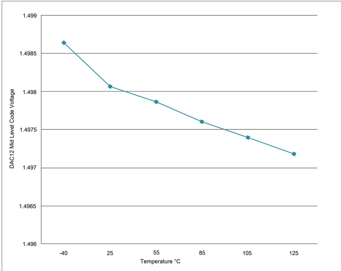
**Figure 30. Offset at half scale vs. temperature**
