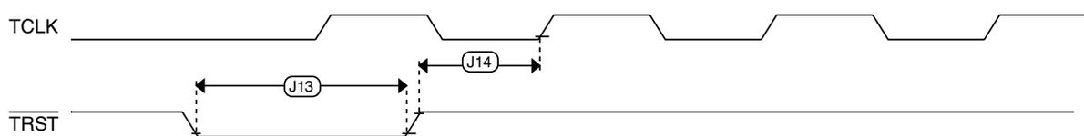
Figure 23.  $\overline{\text{TRST}}$  timing
