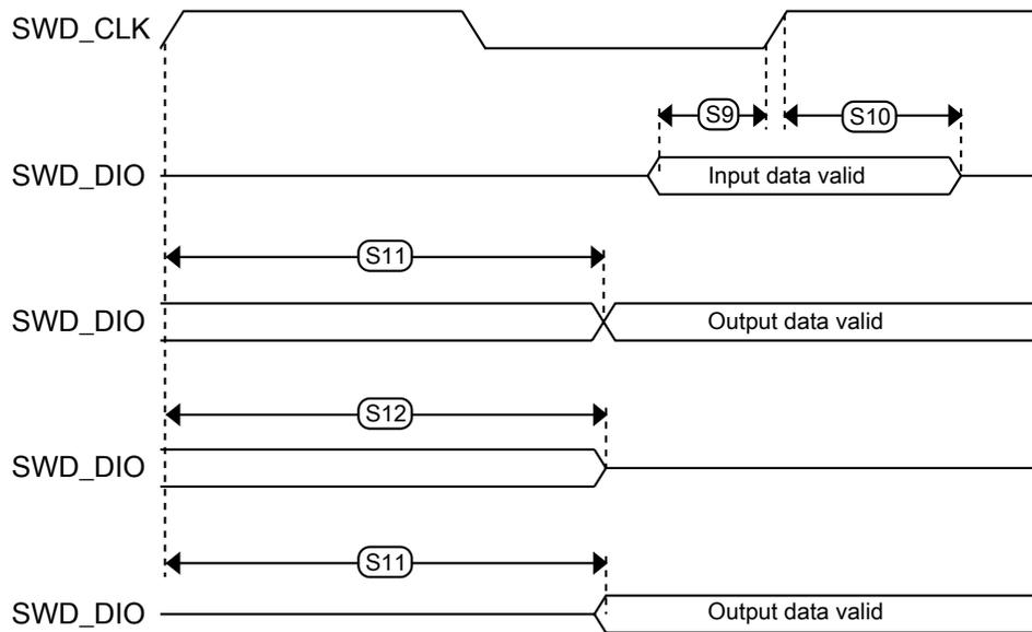
Figure 19. Serial wire data timing
