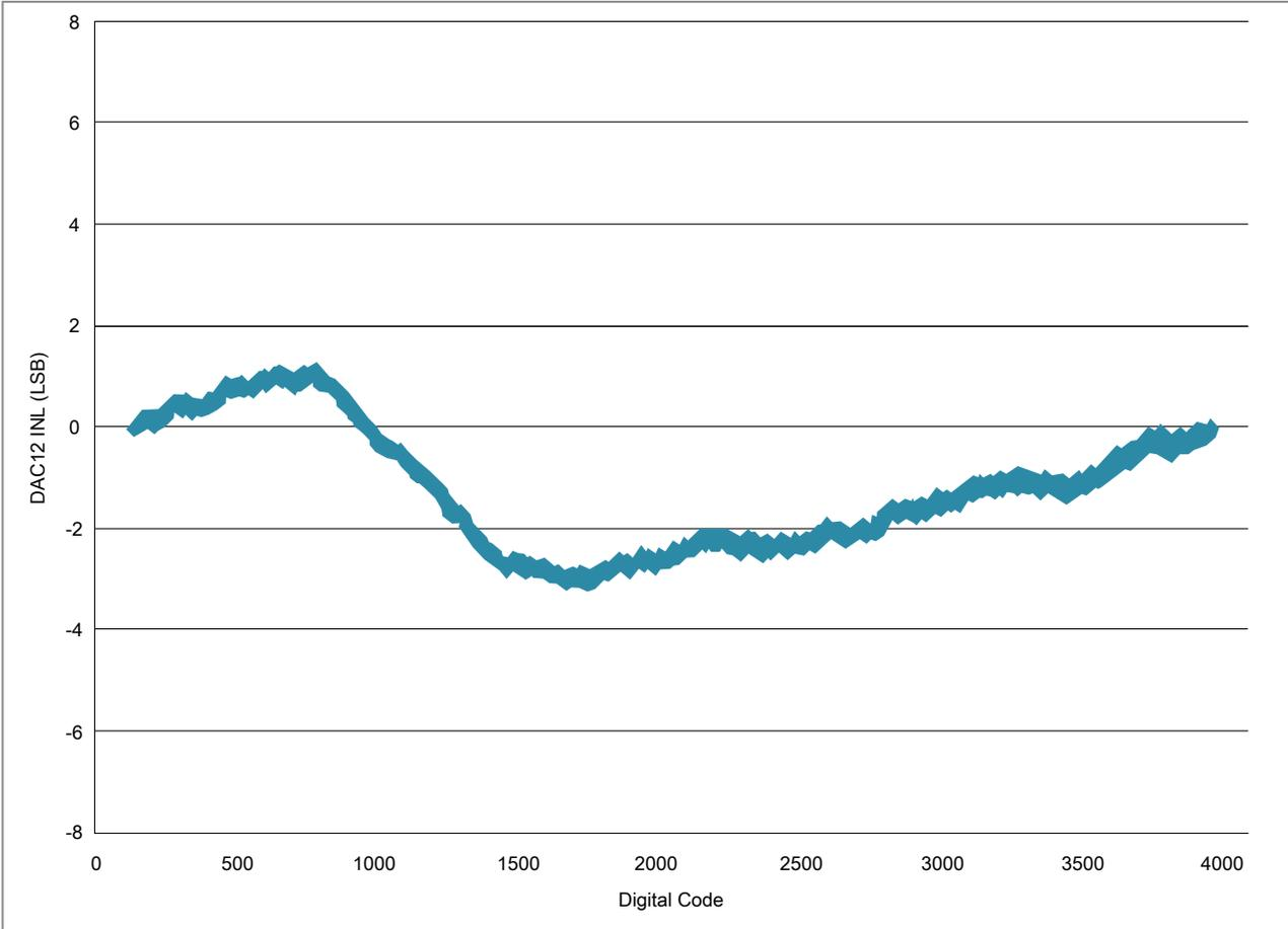
Figure 29. Typical INL error vs. digital code
