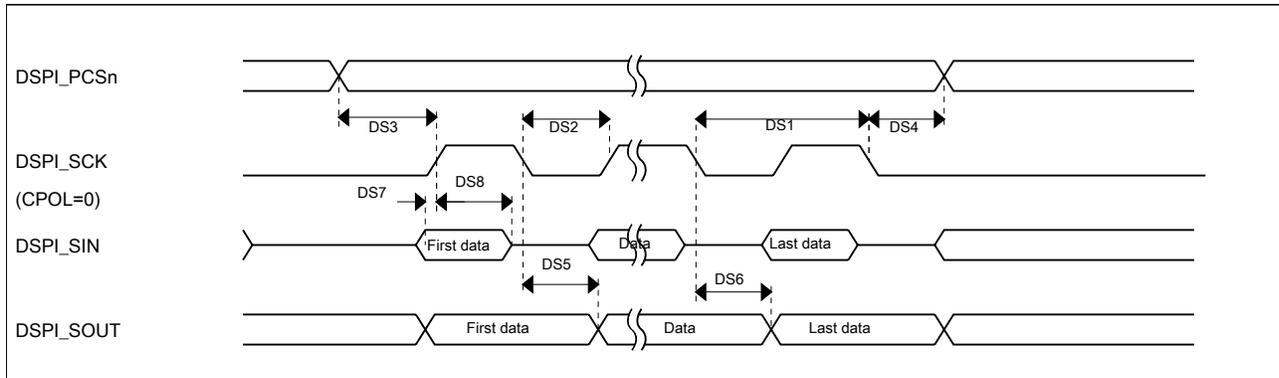
Figure 31. DSPI classic SPI timing — master mode
