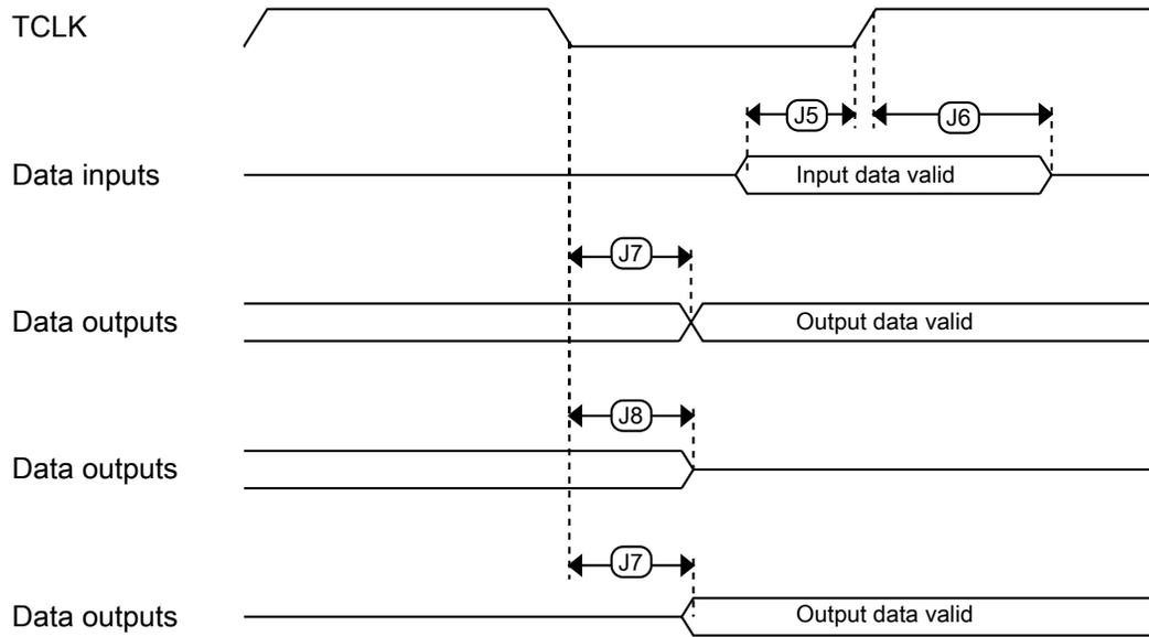
Figure 21. Boundary scan (JTAG) timing
