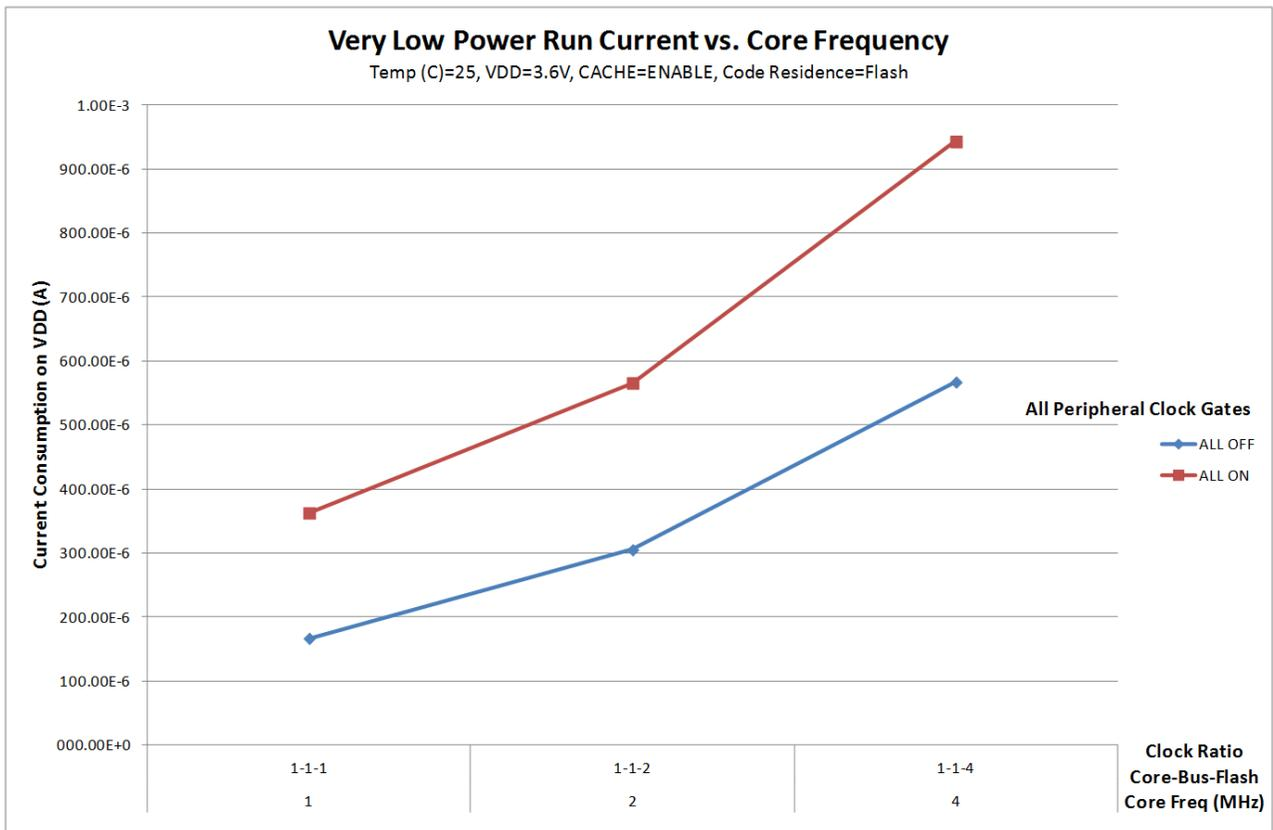
**Figure 17. VLPR mode supply current vs. core frequency**
