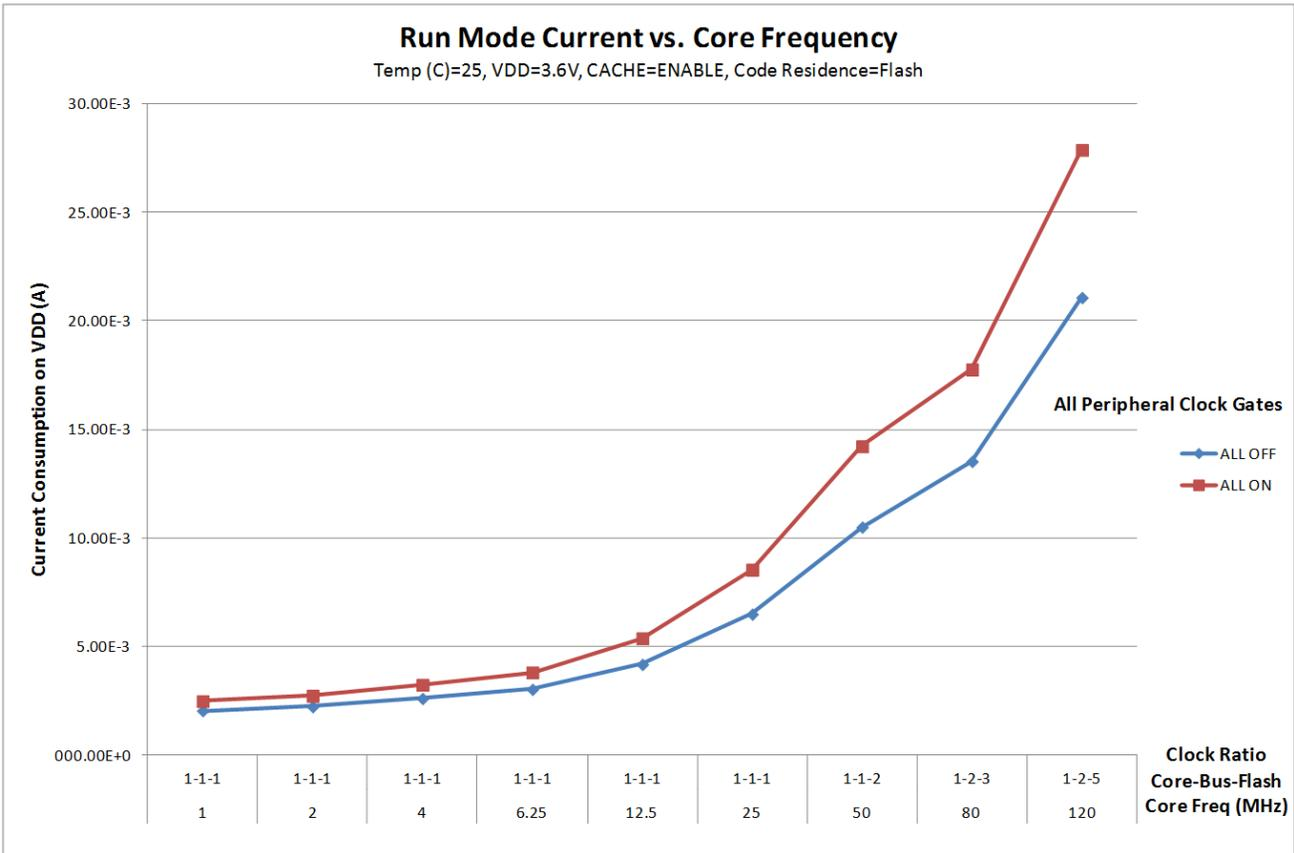
Figure 16. Run mode supply current vs. core frequency
