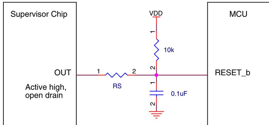
**Figure 44. Reset signal connection to external reset chip**
