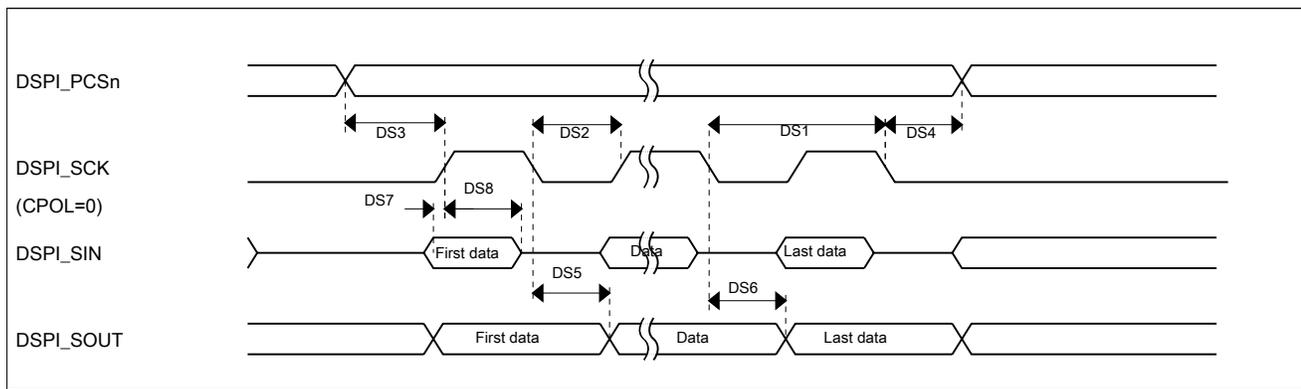
**Figure 33. DSPI classic SPI timing — master mode**
