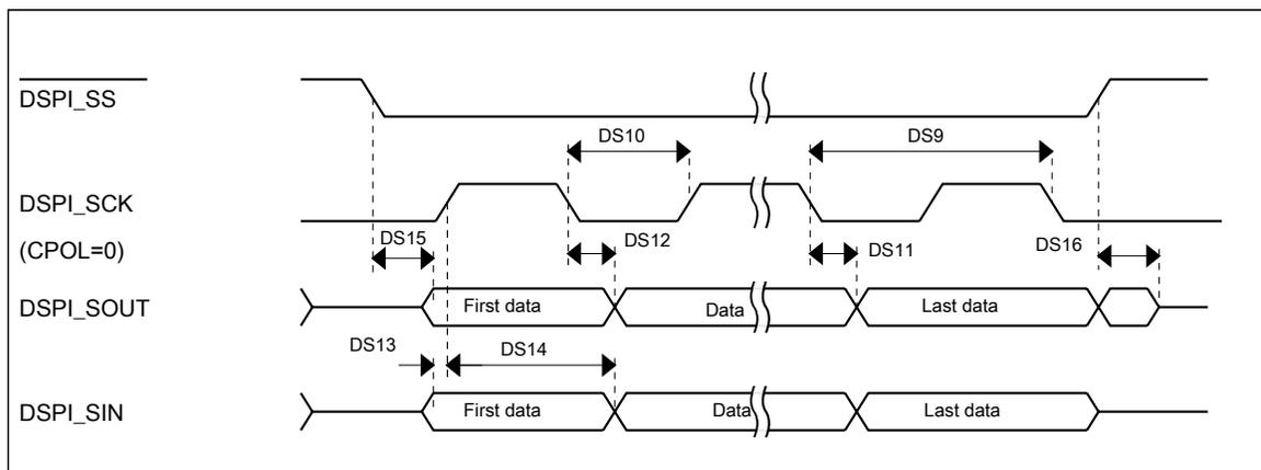
Figure 32. DSPI classic SPI timing — slave mode
