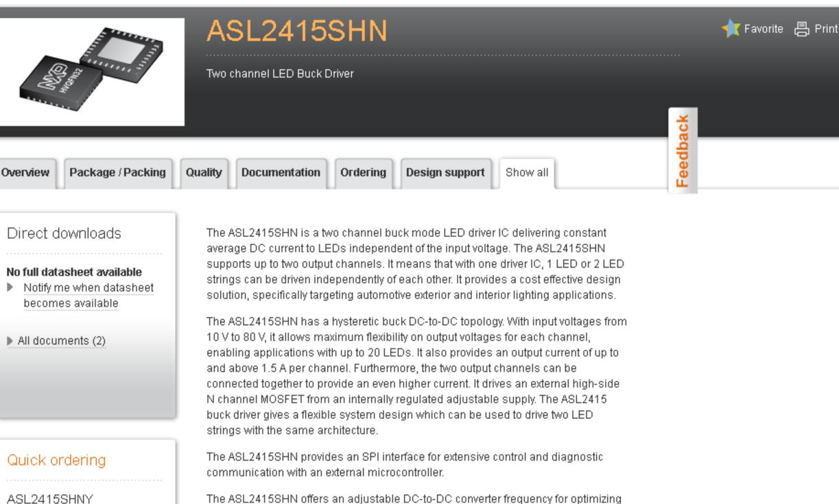
condition. This site uses cookies. Why? Click here to find out more. Close 🗵 The device is housed in a very small HVQFN32 pin package with an exposed thermal pad and is designed to meet the stringent requirements of automotive applications. It is fully AEC Q100 grade 1 qualified. It operates over the -40 °C to
