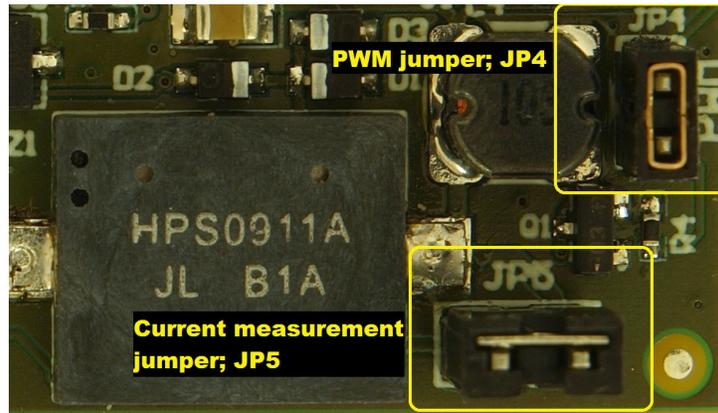
Figure 5. Buzzer connected to PWM through a jumper
