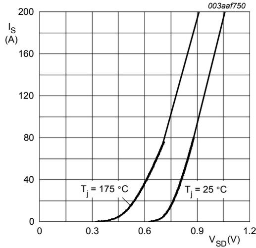
Fig. 17. Source (diode forward) current as a function of source-drain (diode forward) voltage; typical values
