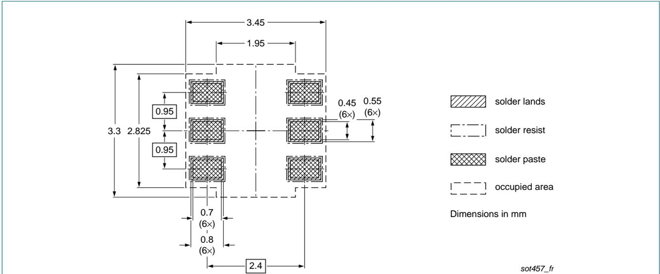
Fig 19. Reflow soldering footprint for SOT457 (TSOP6)
