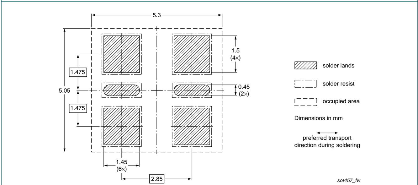
Fig 20. Wave soldering footprint for SOT457 (TSOP6)
