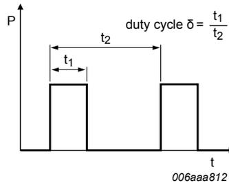
Fig. 31. Duty cycle definition
