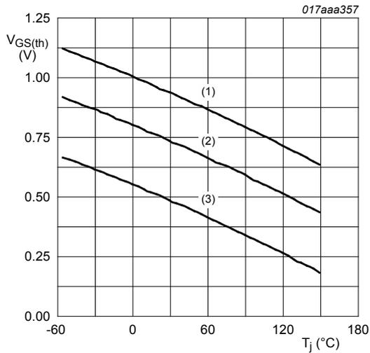
$I_D = 0.25\text{ mA}; V_{DS} = V_{GS}$
