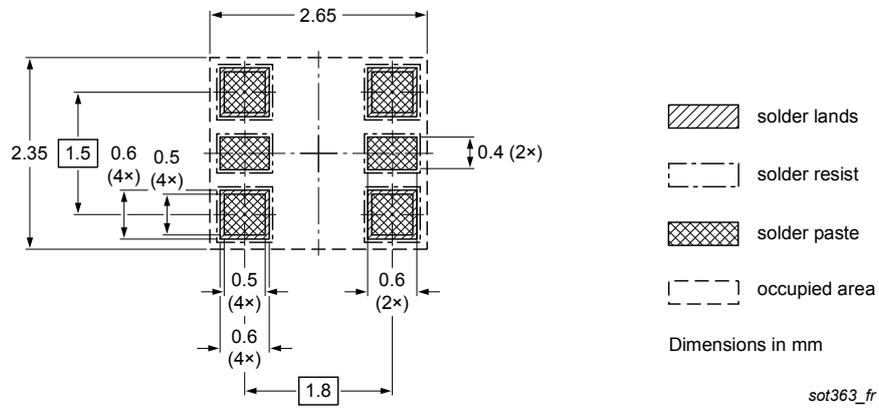
Fig. 33. Reflow soldering footprint for TSSOP6 (SOT363)
