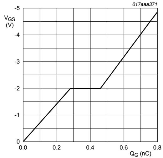
$I_D = -0.4 \text{ A}; V_{DD} = -10 \text{ V}; T_{amb} = 25 \text{ }^\circ\text{C}$
