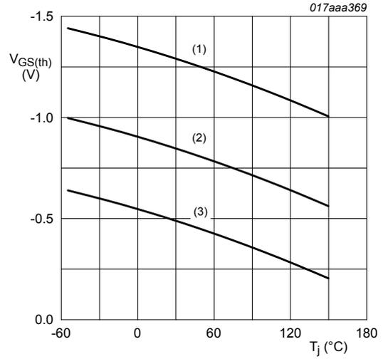
$I_D = -0.25 \text{ mA}; V_{DS} = V_{GS}$
