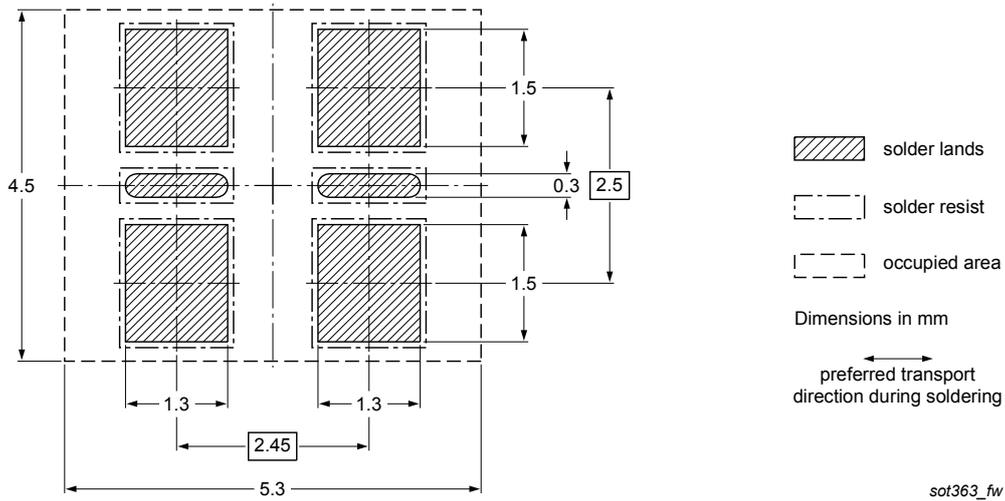
Fig. 34. Wave soldering footprint for TSSOP6 (SOT363)
