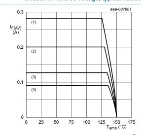
FR4 PCB, mounting pad for cathode 1 cm<sup>2</sup>  $T_i = 150$  °C
