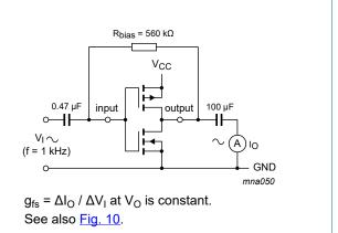
Fig. 9. Test set-up for measuring forward transconductance
