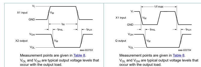
Fig. 5. Input X1 to output X2 propagation delay times
