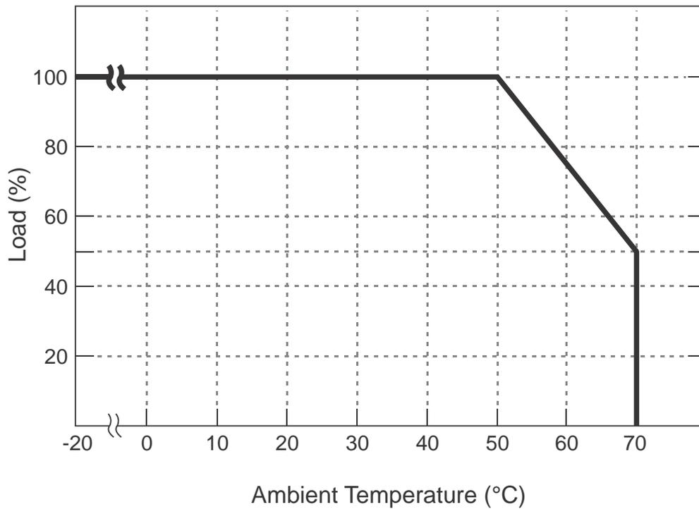
**Figure 3-1 Derating Curve: Models DL10 thru DL100 Series**
