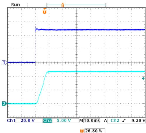
Start-up Delay ( $V_{in} = 48V$ ,  $I_{out} = 20A$ ,  $C_{load} = 5000\mu F$ ,  $T_a = +25^{\circ}C$ ) Ch1 = Vin, Ch2 = Vout
