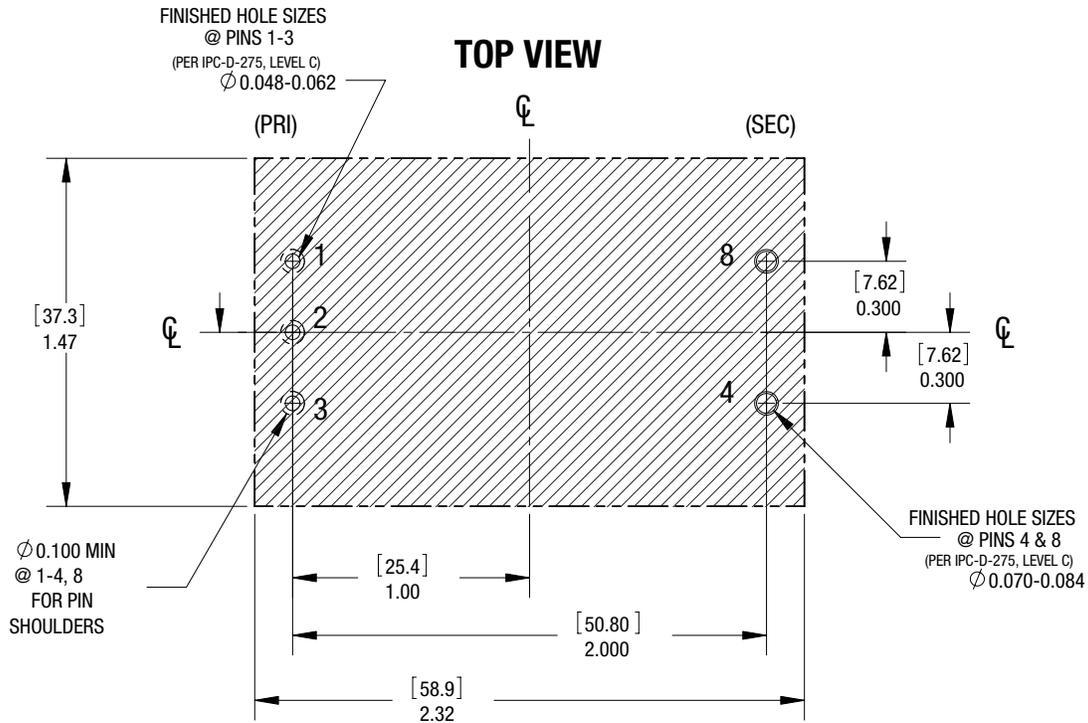
It is recommended that no parts be placed beneath converter (hatched area).
