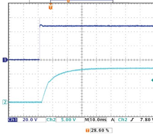
On/Off Enable Delay (Vin=48V, Vout=nom, Iout=20A, Cload=5000µF, Ta=+25°C)
