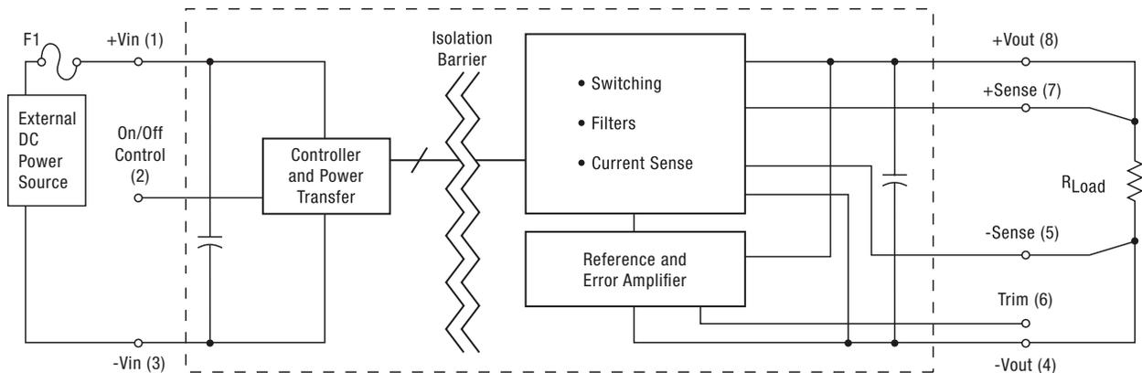
Figure 1. Connection Diagram
