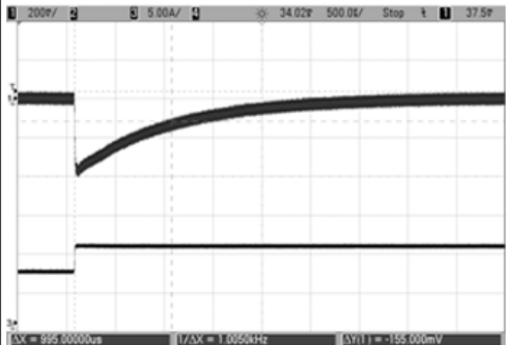
Step Load Transient Response (Vin = 48V, Vout = nom, Cload = 1μF || 10μF, Iout = 50 to 75 to 50% of full load, Ta = +25°C) Ch1 = Vout, Ch2 = Iout.
