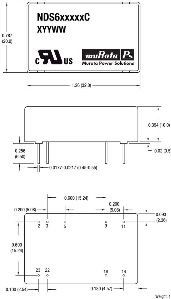
All dimensions in mm (inches)  $\pm 0.5$  (0.020) except pin to pin tolerance  $\pm 0.25$  (0.010).
