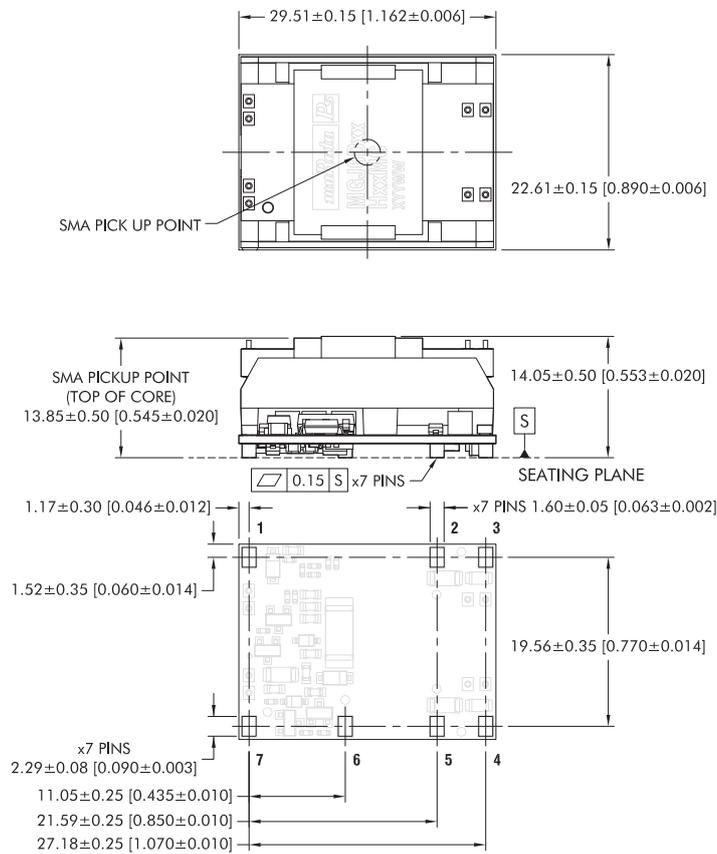
All dimensions in mm (inches), Controlling dimensions is mm.
