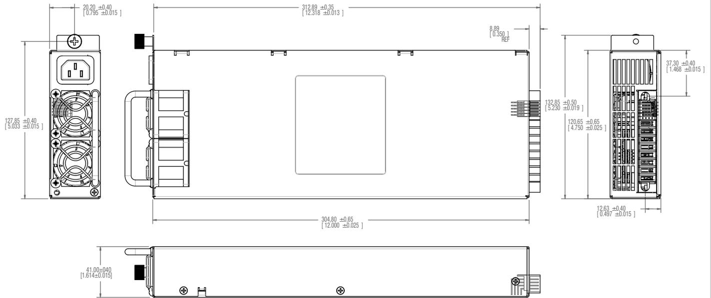
AC Input Connector: The AC input connector is standard IEC320 C14 (15A).
