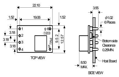
[unit: mm] Tolerance: 0.25mm
