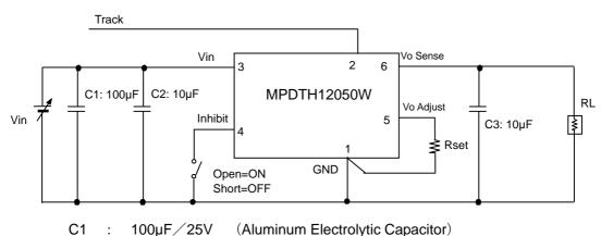
C1 :  $100\mu F/25V$  (Aluminum Electroly C2 :  $10\mu F/25V$  (Ceramic Capacitor) C3 :  $10\mu F/6.3V$  (Ceramic Capacitor)
