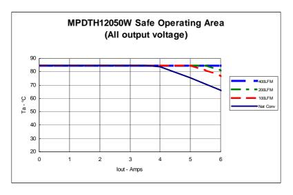
The above SOA represents the condition at which internal components are at or below the manufacturer's maximum operating temperatures. Derating limits apply to modules soldered directly to a 4 in.x4in. 4-layer PCB with 1 oz. copper. For more reliable operation, appropriate derating is desirable.
