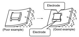
(2) Components location on PCB separation
