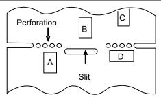
\*1 A > D is valid when stress is added vertically to the perforation as with Hand Separation. If a Cutting Disc is used, stress will be diagonal to the PCB, therefore A > D is invalid.
