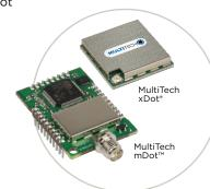
The mDot and xDot are LoRaWAN compliant,
