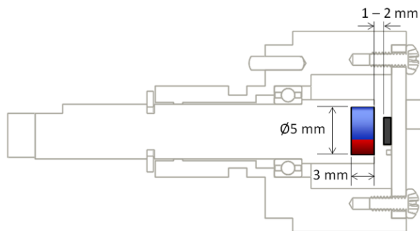
Figure 5: Example of Potentiometer-Like Assembly
