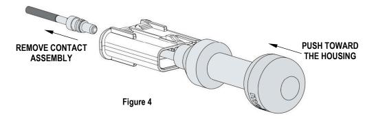
**Note:** After the terminal contact is extracted, inspect the housing cavity to determine if any damage was done to the housing.
