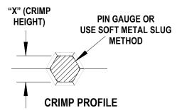
Use gauge pins or soft metal slug (solder) method to measure the "X" dimension. Verify the tooling crimp height calibration by referring to the Go/No Go dimensions shown in the chart below.
