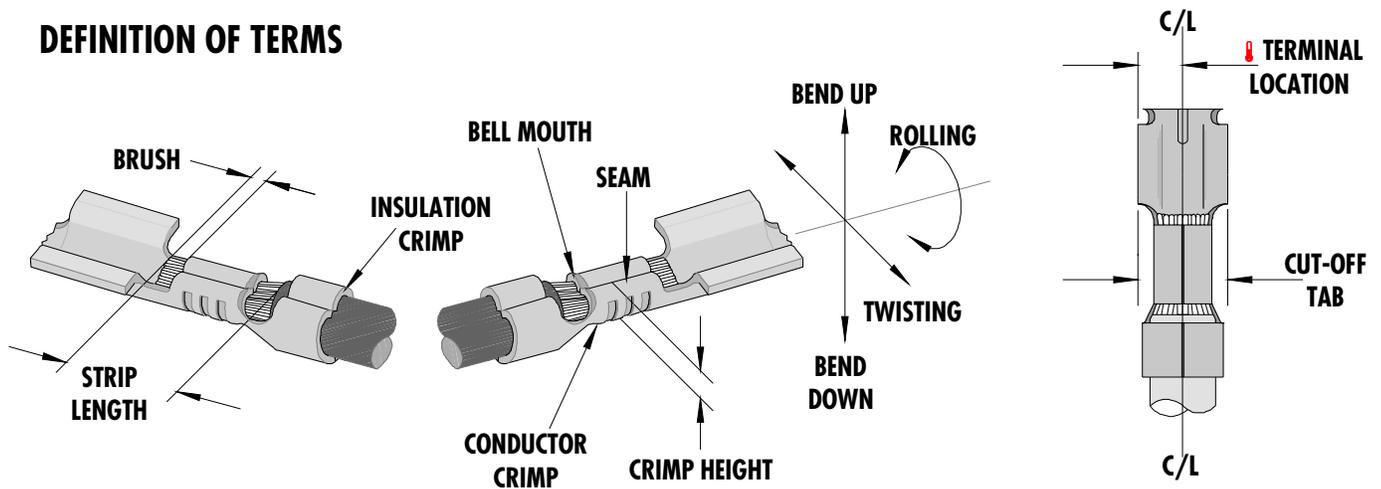
Terminal is to be centrally located between the two (2) cut-off tab edges by one half of the total cut-off tab tolerance. This illustration is a generic terminal representation and not an exact image of any terminal listed in the scope.
