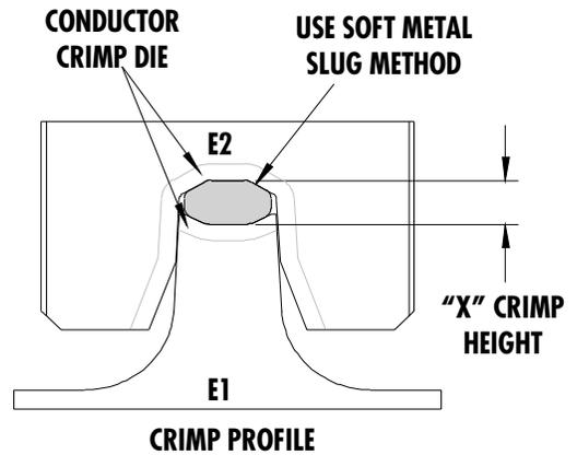
Use soft metal slug (solder) method to measure the "X" dimension. Verify tooling crimp height calibration by referring to the Go/No Go dimensions shown in the chart below.
