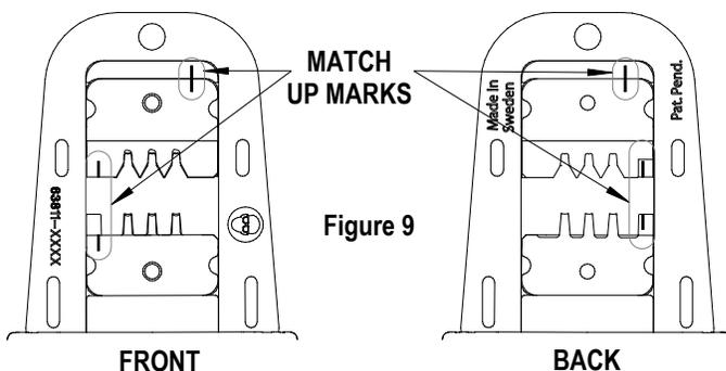
4. Do the same thing with the lower tooling and tighten the M3 screws. Be sure the small markings line up.
