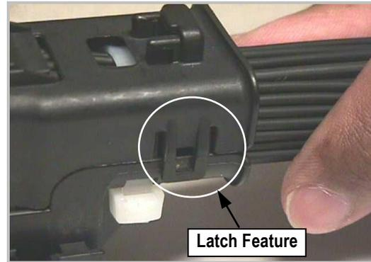
2. With wire dress cover latch features unlatched; insert finger into wire dress cover and pull up and away from the wire bundle.
