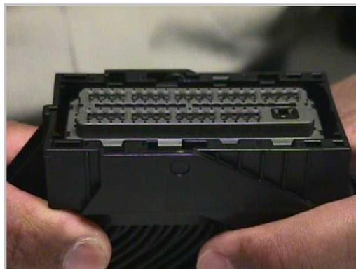
1. With the terminal fully installed, the TPA can be seated into its final-lock position by applying an even force to both ends until it comes to a stop. If the TPA resists it may be detecting a partially installed terminal.
