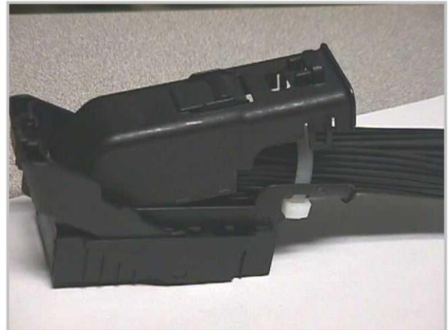
3. At this time the tie wrap should be removed from the wire bundle for easier access to the wire to be serviced.
