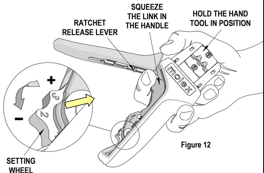
1. Hold the hand tool in the palm of your hand as shown in Figure 10. Using the index finger squeeze the link towards the top of the hand tool frame. This will release the preload adjustment wheel.
