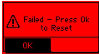
If the foot switch cable is connected to the crimp force monitor, the foot switch will be disabled when a fail occurs. Pressing a keypad button will silence the alarm and re-enable the foot switch.
