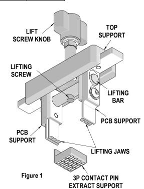
In order for this tool to function, there is a "Keep-Out Zone" of .197" (5.00mm) around the header that needs to be clear of other components. See Figure 2. This is a general requirement, regardless of the header being removed.
