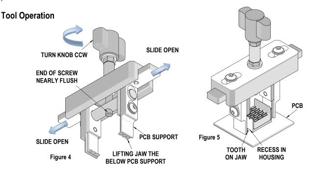
**Note:** Some longer-length headers may need the following steps repeated, with the tool being re-applied along the length of the assembly
