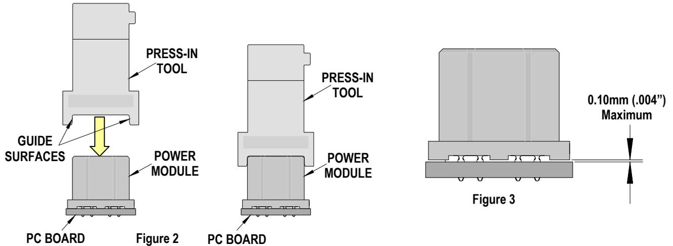
3. Using the application tool and an appropriate press, seat the vertical power module until there is less than 0.10mm (.004 in) clearance between the bottom of the plastic housing and the surface of the PCB. See Figure 3.
