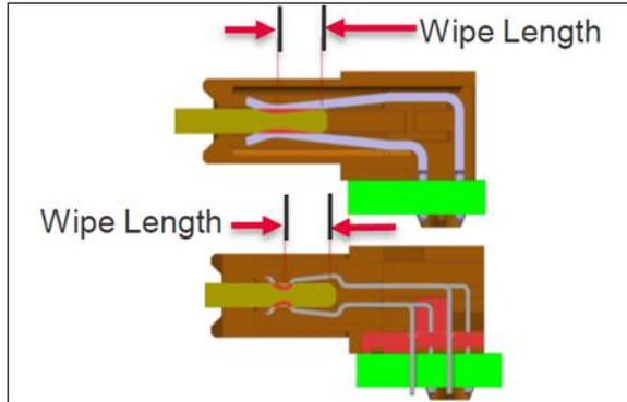
**Final position/fully mated condition (LPH Power & Signal):**
