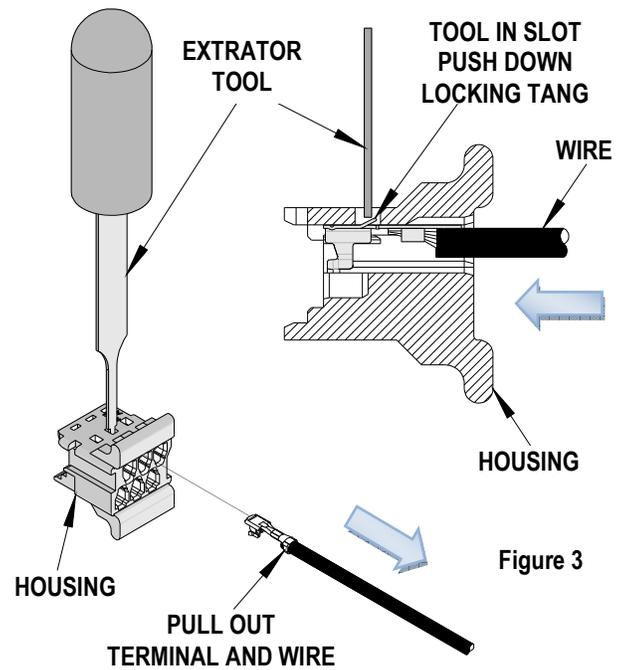
**CAUTION:** This extractor tool should be used to extract the terminal only. Using it for unintended purposes may cause injury or damage to parts. Be careful not to deform the end of the terminal.
