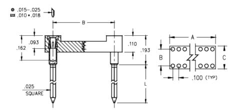
**Description:** DIP Socket Wrapost Tail 4 Level Wrapost Tail Open Frame Accepts .015-.025" Leads Plating Code: 93 Shell Plating: 200 μ" Tin/Lead(93/7) over 100 μ" Nickel Inner Contact Plating:
