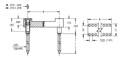
Description: DIP Socket Wrapost Tail 4 Level Wrapost Tail Open Frame Accepts .015-.025" Leads Plating Code: 93 Shell Plating: 200 μ" Tin/Lead(93/7) over 100 μ" Nickel
