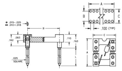
**Description:** DIP Socket Integral Decoupling Capacitor 2 Level Wrapost Tail Open Frame Accepts .015-.025" Leads
